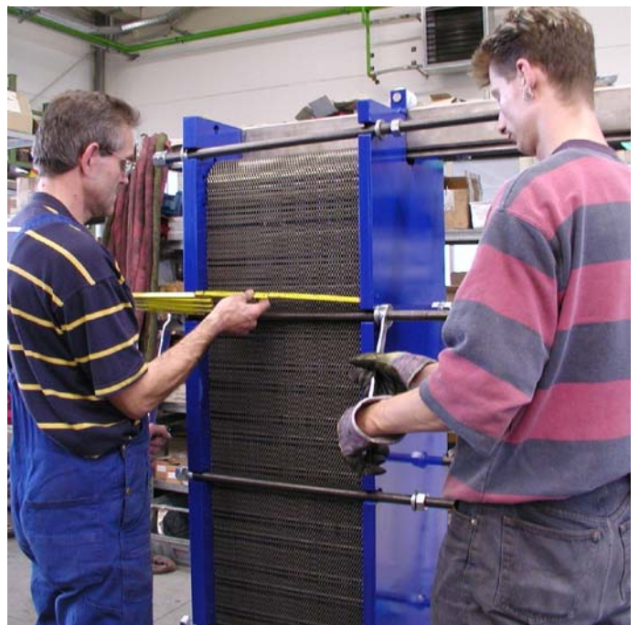
Figure 15: Correct opening of the PHE and check of allowed inclination of the pressure plate.
